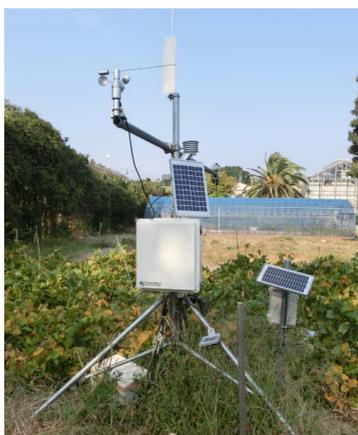
*Fig. 2. A weather station for meteorological measurements in a soybean field*
