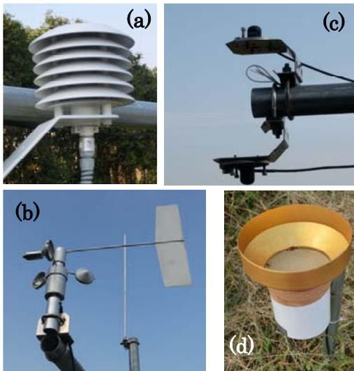
Fig. 3. Meteorological measurements at the weather station: (a) air temperature and relative humidity sensors, (b) an anemometer for wind speed and direction, (c) pyranometers for incoming and reflected solar radiations and (d) a rain gage
