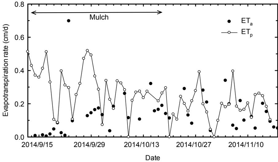
Fig. 6. Potential evapotranspiration rate according to the Penman-Monteith combination equation ( $ET_p$ ) and actual evapotranspiration rates based on the water mass balance ( $ET_a$ )
