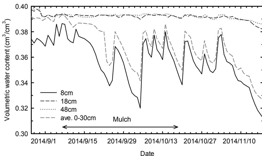
Fig. 5. Volumetric water content variations at three depths measured with horizontally installed TDR probes, and averaged water contents for 0 - 30 cm depth measured with a vertically installed TDR probe
