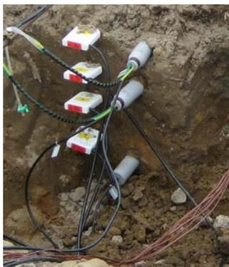
*Fig. 1. TDR probes and tensiometers horizontally installed in a soil profile*
