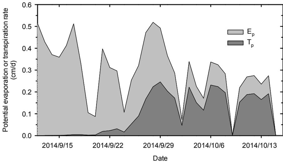
Fig. 7. Potential evaporation ( $E_p$ ) and potential transpiration rate ( $T_p$ ) derived from partitioning of potential evapotranspiration ( $ET_p$ )
